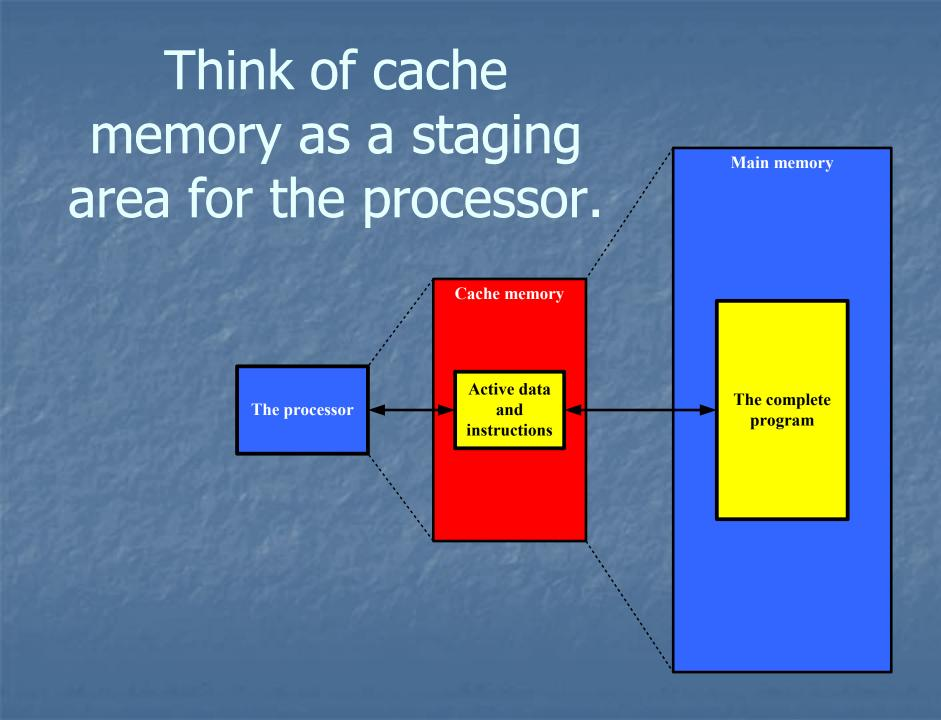
The processor manipulates the data stored in memory under the control of a program stored in the memory.
