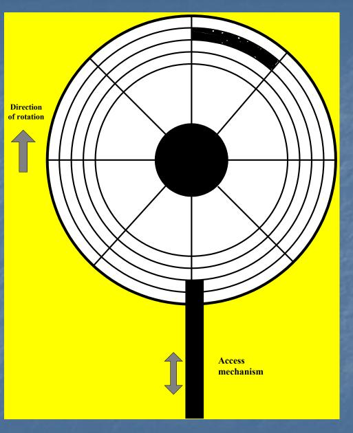
b. The system waits while the sector rotates to the read/write head, causing rotational delay, and the data is transferred into memory.
